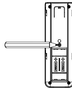
If teaching-in was successful, the device LED (**B**) of the switch actuator will flash green for one second. If teaching-in failed, the device LED will light up green for two seconds. In this case, please try again.
