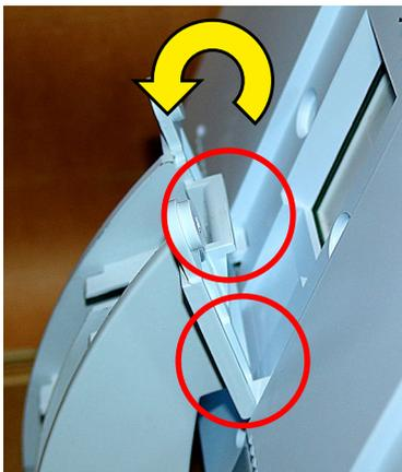
4. Attach the weather station to the clips on the base support and swivel it onto the base support until the screw domes sit properly in the corresponding receptacles on the weather station.
