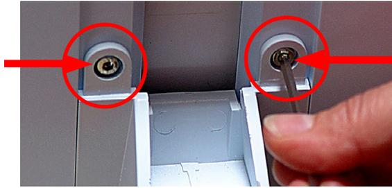
5. Use the hexagon wrench and two hexagon socket screws supplied to screw the base support onto the weather station.
