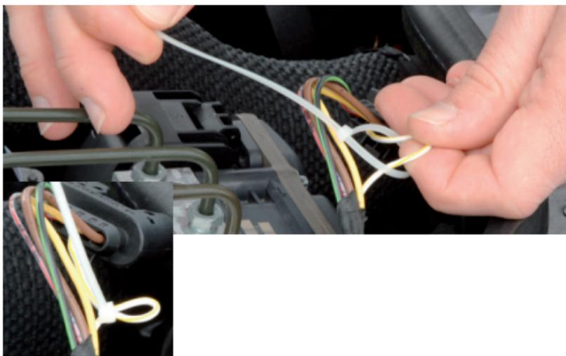
The wire needs to be at least a few centimetres in length to allow you to twist it even once. Do not pull forcefully on the wire. It may be necessary to find another installation location with a longer wire in order to obtain the length you need.
