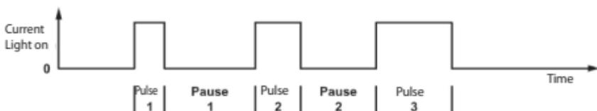
When flashing sequences are being set, the headlight flasher sensor is able to store the times for 5 pulses and pauses plus a tolerance value separately for each of its two channels. An individual sequence can be set for each of the two channels. These sequences are channel parameters which can also be set in the Web UI (if available).
