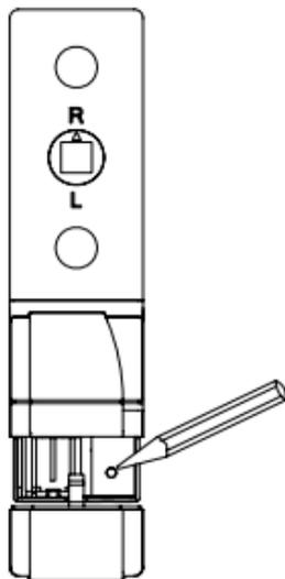
To actuate teach mode on the window rotary handle sensor, press the teach button with a pointed object. The device LED flashes orange. (Abort with a short press of the teach button, the device LED will then illuminate in red.)
