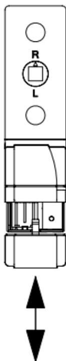
Push the battery compartment cover (arrow) downward and then remove it. Insert the two LR44 batteries provided with proper polarity according to the polarity markings into the battery compartment. The batteries are held in the battery compartment by the tension on the battery caused by the contacts.
