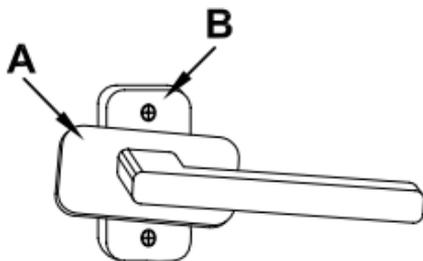
If deformations should appear on the square shaft of the window handle (caused by mechanical stress, see ! in the following figure), remove these with a file.
