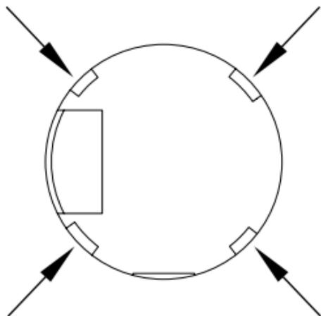
Insert the provided Lithium battery (CR 2032), with correct polarity in accordance with the polarity markings in the battery cabinet (E) (positive pole at top).
