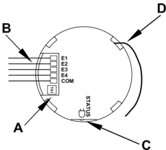
To actuate teach mode on the push-button interface, press the teach button with a pointed object. The push-button interface is then in configuration mode, indicated with a flashing green device LED. (If you want to exit configuration mode, press the teach button again.)
